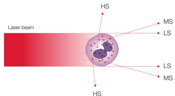
**Figure 2.** Swelab Lumi uses laser-based flow cytometry for WBC, with separate channels for 4-part and BASO differential. Low angle signal (about 1° to 5°) represents the cell volume information, middle angle signal (about 7° to 20°) represents the cell nucleus information, high angle signal (about 90°) represents the cell nucleus and cytoplasm information.
