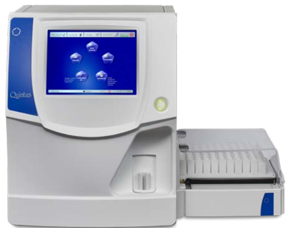
Fig 1. Quintus 5-part hematology analyzer equipped with optional autoloader unit.
