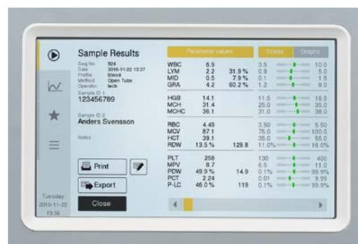
**Figure 1.** MPA function offers fast pre-donation testing. (A) Take a finger-stick blood sample. (B). The MPA adapter lets you analyze capillary samples directly and saves the vein for donation. (C) In one minute, key results can be viewed on the touchscreen.
