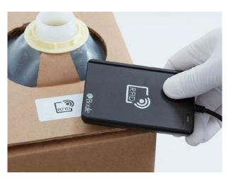
To ensure analytical quality and performance of your Boule hematology system, use the designated reagents that are entered by scanning the RFID card on the container.
