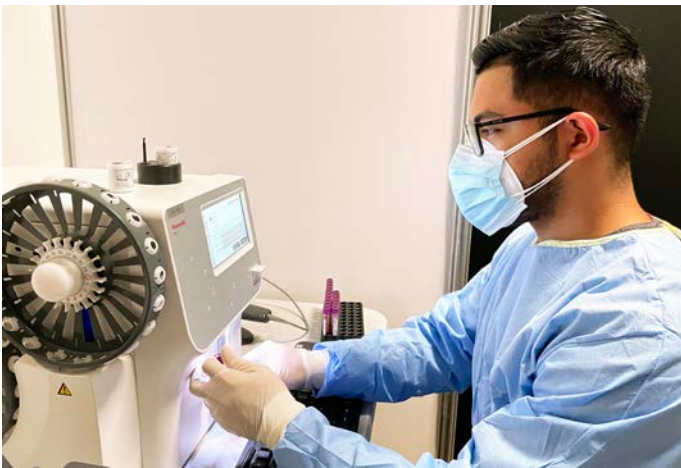
Fig 5. Dr. Bonilla uses a Swelab Alfa Plus analyzer equipped with space-saving automation wheels to cope with high workloads, and with the MPA inlet that reports a full CBC from a finger-stick sample in about one minute.
