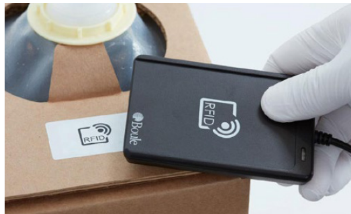
Fig 7. To ensure analytical quality and performance of the hematology system, it is recommended to only use the designated reagents that are entered by scanning the RFID card (or barcode) on the container.
