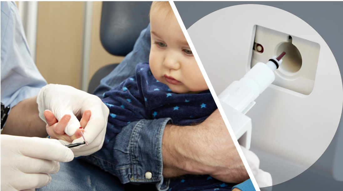
Fig 1. Boule hematology analyzers equipped with the micro-pipette adapter (MPA) inlet allow for CBC testing directly from a finger-stick blood sample taken directly from the patient. No vacuum tube, predilution, or tube mixing prior to analysis is required.
