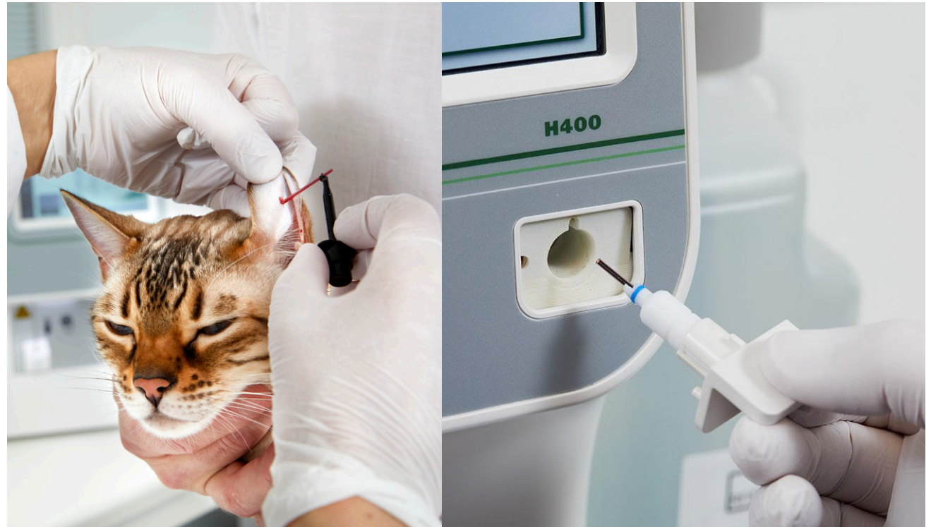
Fig 2. The MPA capillary sample feature of the Exigo H400 is especially suitable for smaller animals such as cats.
