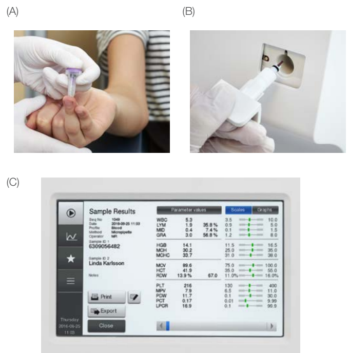
Figure 1. MPA function offers fast pre-donation testing. (A) Take a finger-stick blood sample. (B). The MPA adapter lets you analyze capillary samples directly and saves the vein for donation. (C) In one minute, key results can be viewed on the touchscreen.
