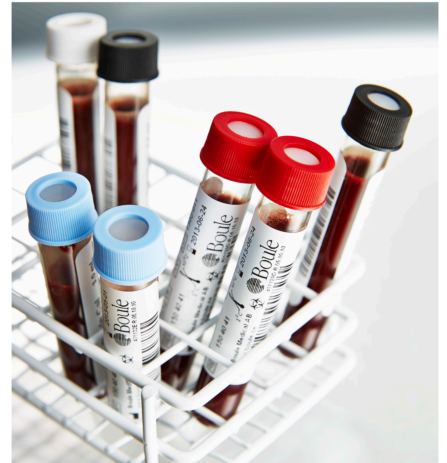
Fig 21. It is recommended to use of Boule controls every day as a routine QC procedure. Barcode screening facilitates input of assay values, while preventing potential errors.
